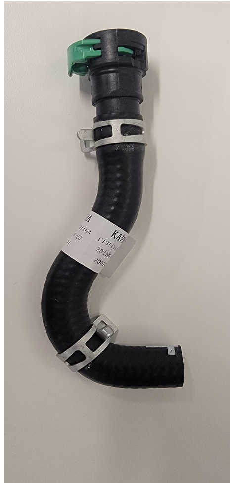
Fuel vapor line from the canister to the DMTL, C131116401104
