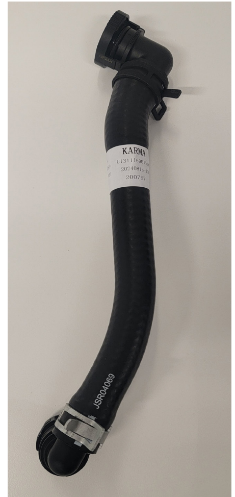
Vent line from the DMTL to FTIV, C131116901504
