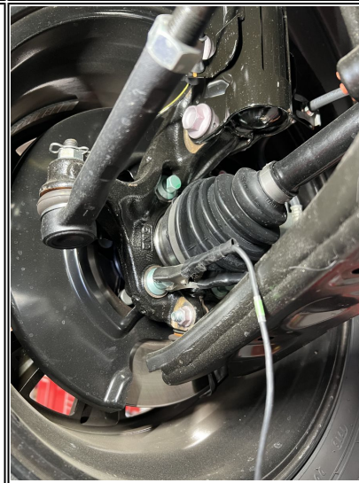
Sensor on wheel bearing bolt.
