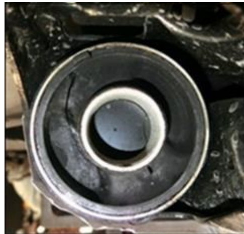
View of Yellow Arrow showing cracked bushing
