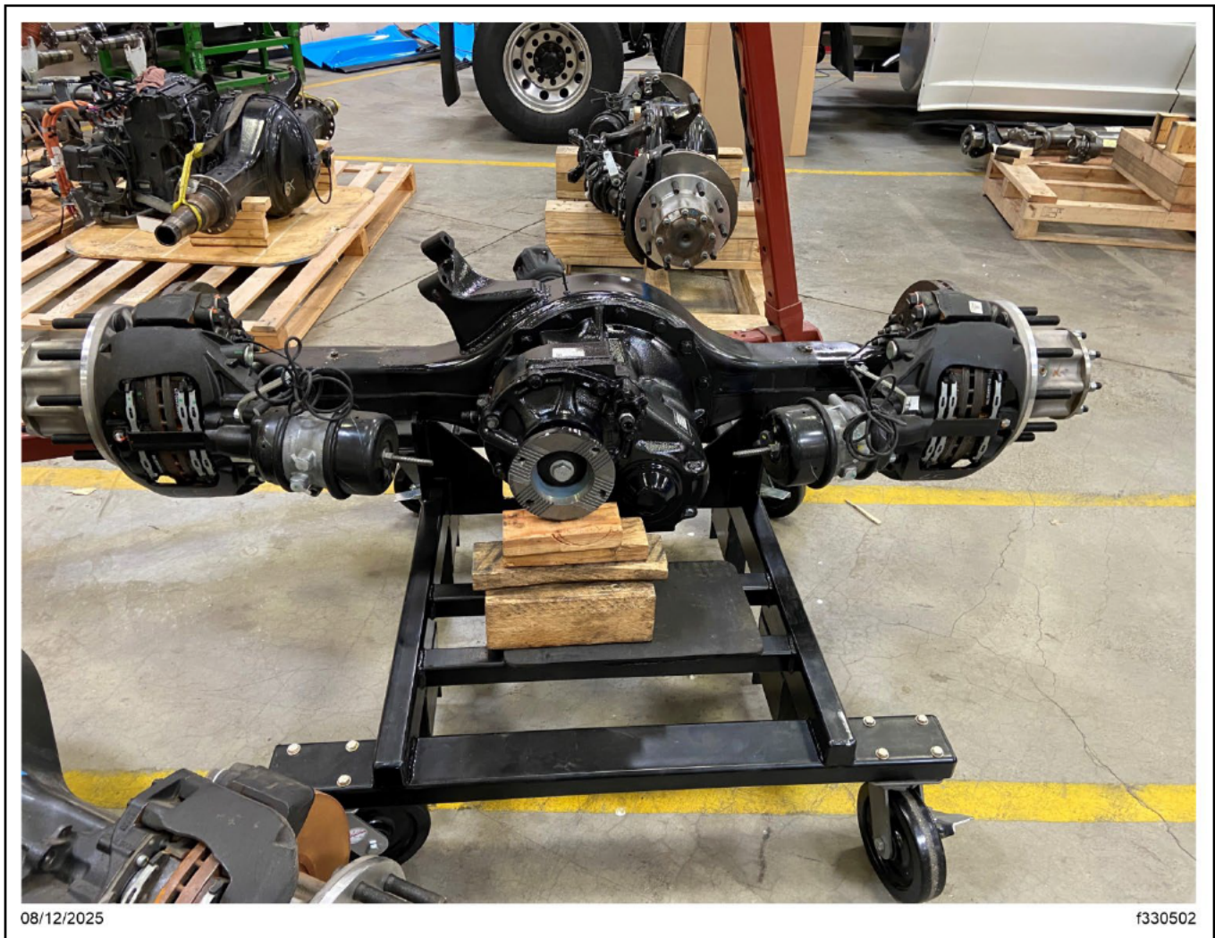
Fig. 4, Axle Removed from the Chassis
