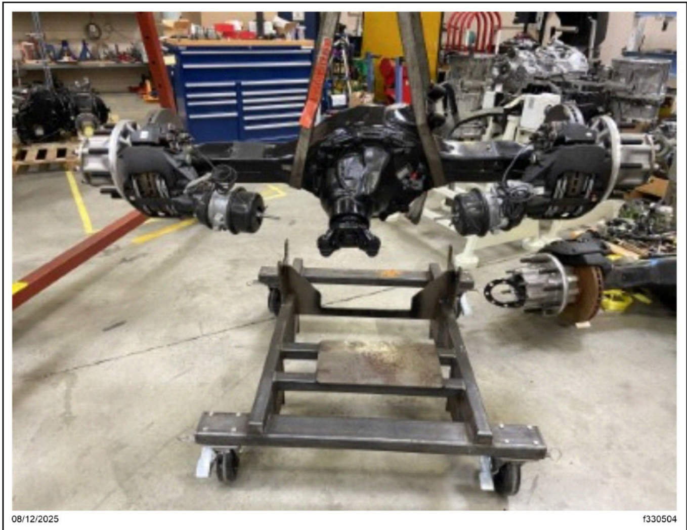
Fig. 6, Craning the New Rear Drive Axle
