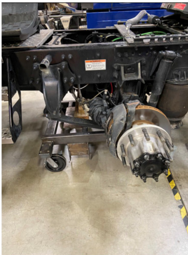
Fig. 1, Resting the Axle on the Dolly
