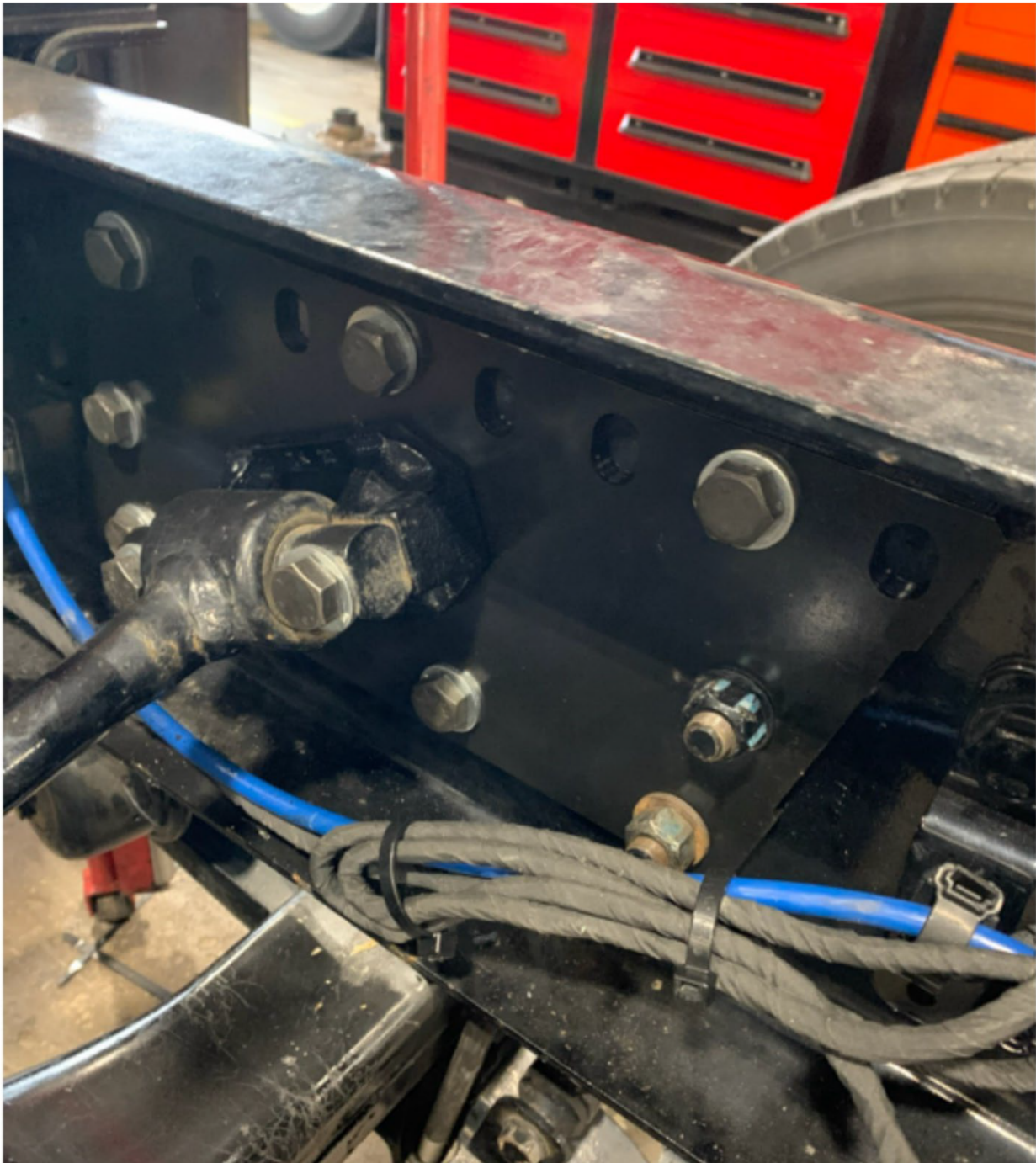
Fig. 7, Left-Hand Forward Lateral Rod and Bolt Installation After Drilling Is Completed
