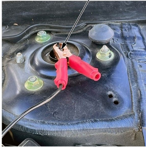
Attach the chassis ear to damper shaft
