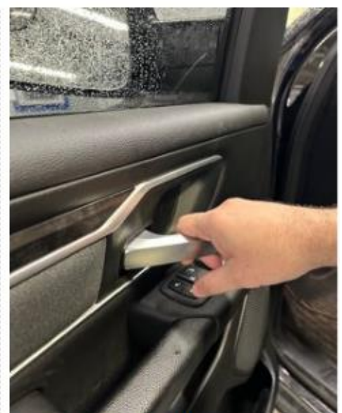
c. Pull Inside Handle to move lock knob to unlocked position.
