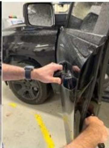
E. While pushing the screwdriver in the catch to open, pull on the outside handle.
