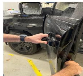
B. While pushing the screwdriver in the catch to open, pull on the outside Handle.
