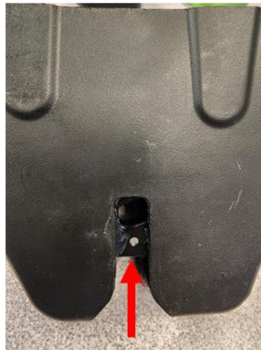
b. Using your finger or a small screwdriver, move the latch into primary position
