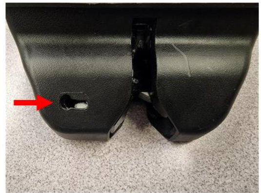
c. Using a small screwdriver, release the latch into full open using the manual keyhole release
