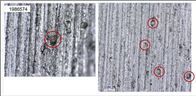
Figure 3. Embedded Aluminum Oxide
