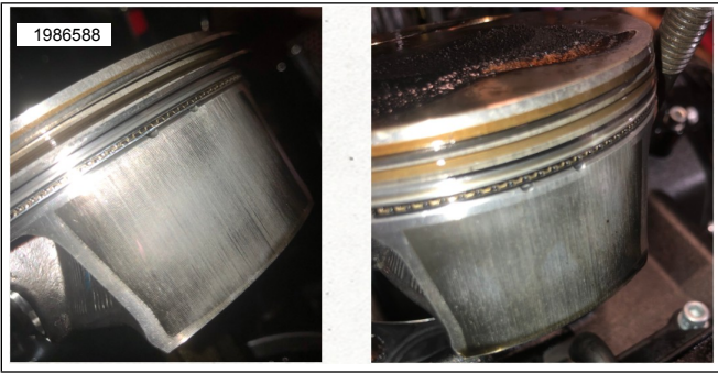
Figure 2. Debris Wear on Piston Rings and Skirts
