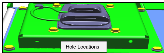
Figure 2: Curb side charge box receptacle face plate location reference.
