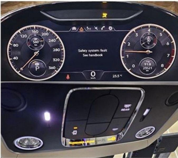
Figure 1. Airbag warning illuminated in the instrument cluster
