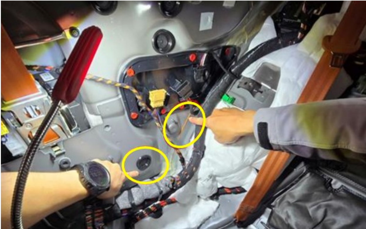
Figure 1. Location of potential leakage
