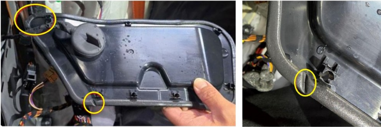
Figure 2. Water shedder with signs of deformation
