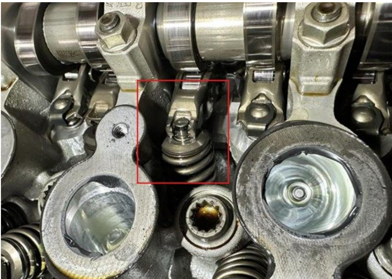
Figure 3. Valvetrain visible wear damage example 2
