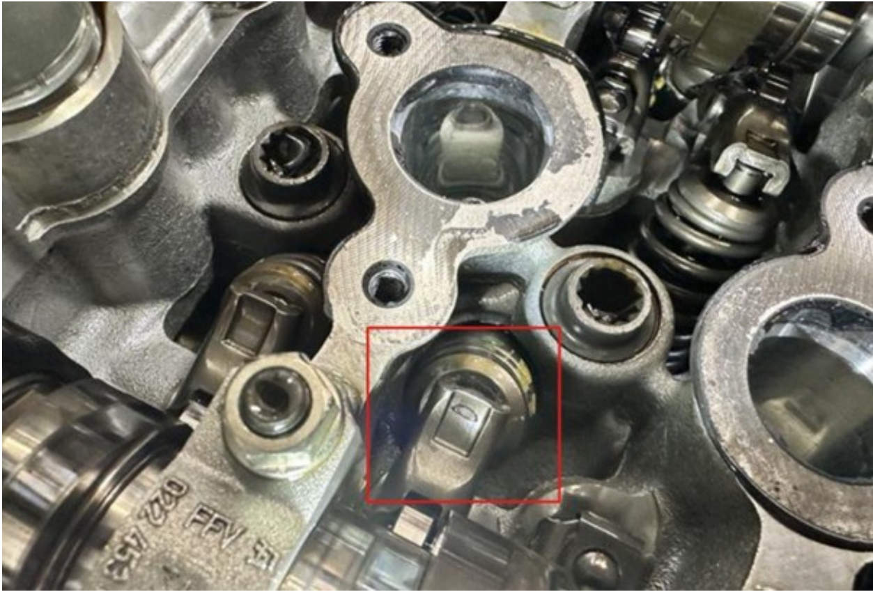
Figure 2. Valvetrain visible wear damage example 1
