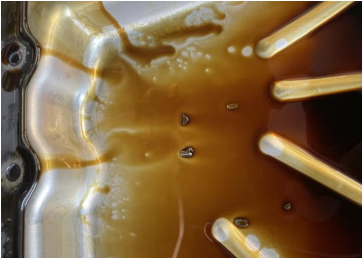
Figure 1. Large debris present in oil example
