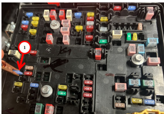
Fig. 1 F08 MOD Cluster Fuse Location
