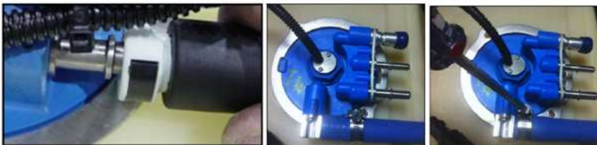
Figure 15: MFHU line installation.
