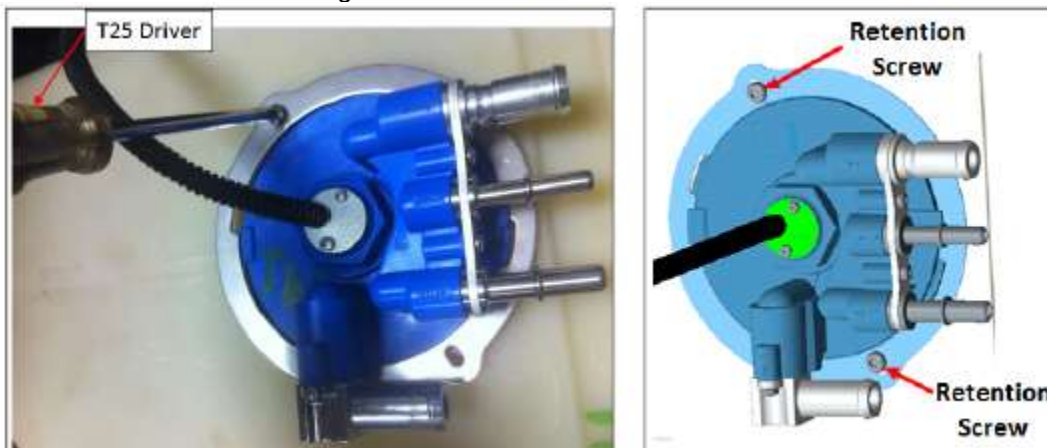
Figure 14: Secure MFHU assembly to the DEF tank with the two retention screws removed in Step 2.
