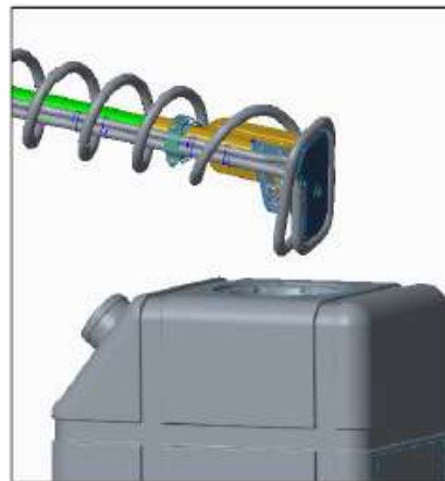
Figure 4: MFHU removal process.
