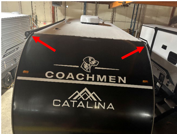
FIG. 1 – LOCATION OF EXTERIOR TRIM PIECES
