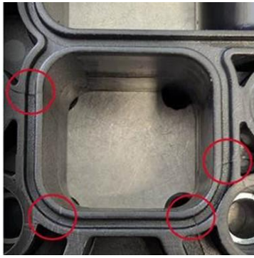
Red circles indicate areas of tooling flash on the manifold
