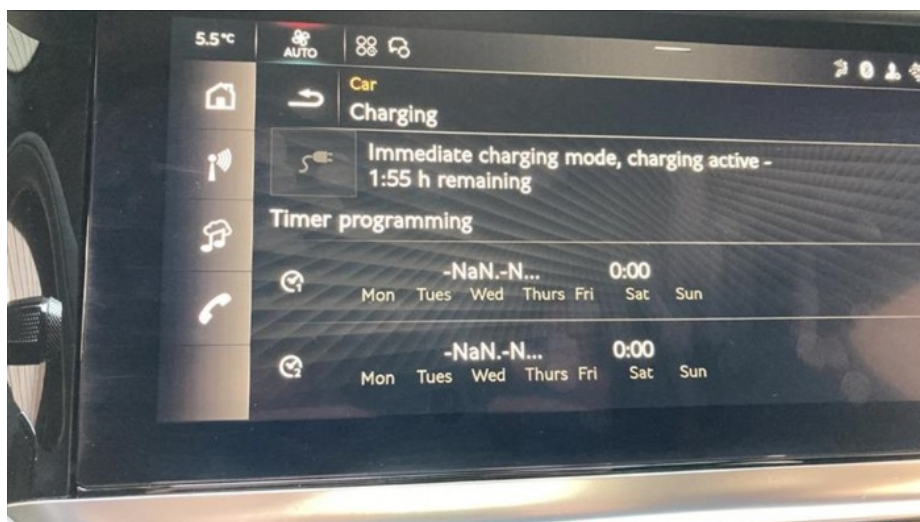
Figure 2. MMI displaying incorrectly set charge timers
