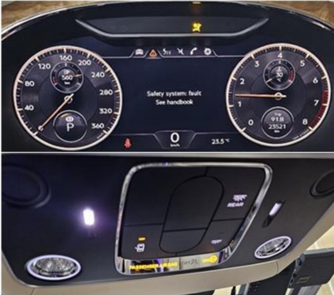
Figure 1. Airbag warning illuminated in the instrument cluster
