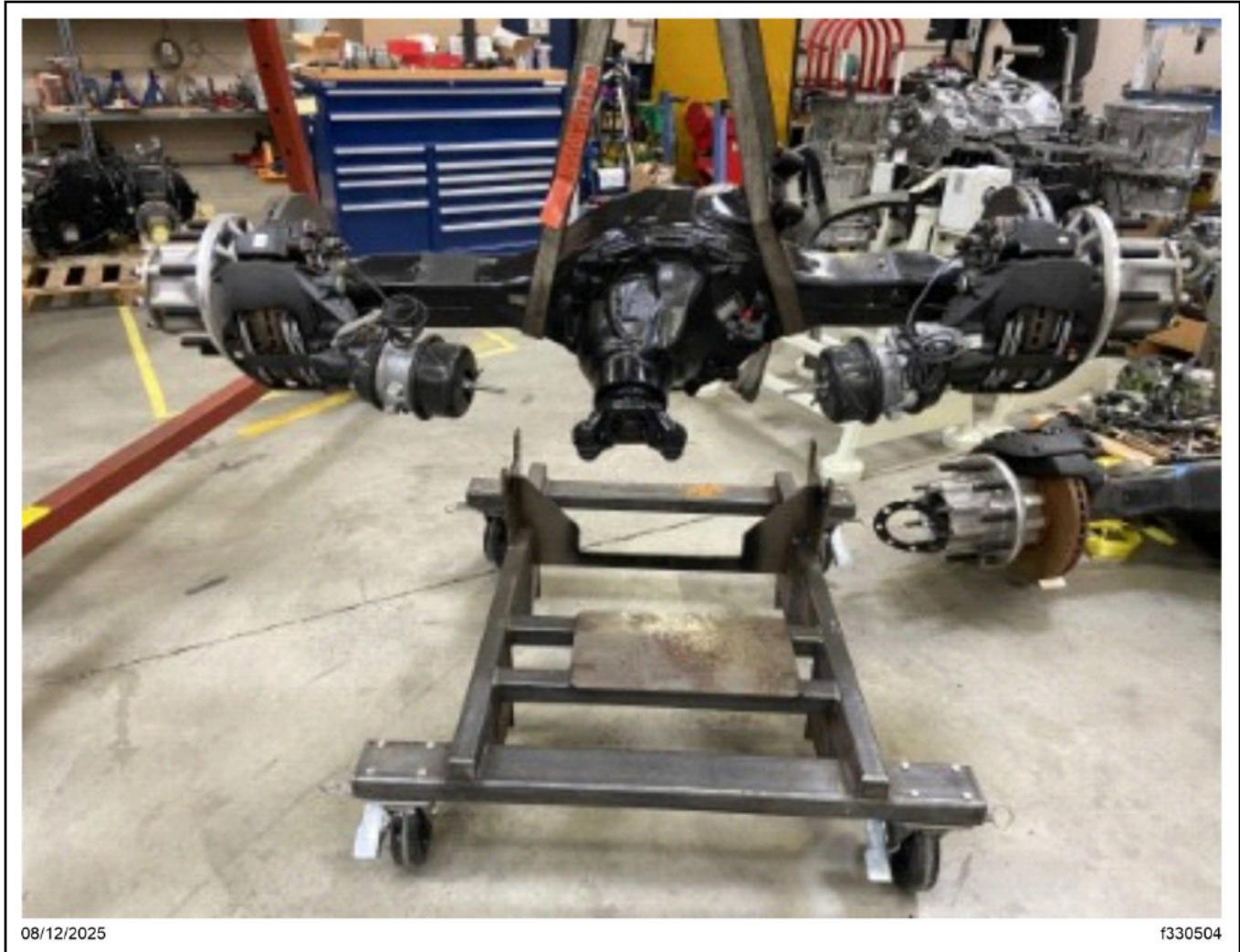
Fig. 6, Craning the New Rear Drive Axle
