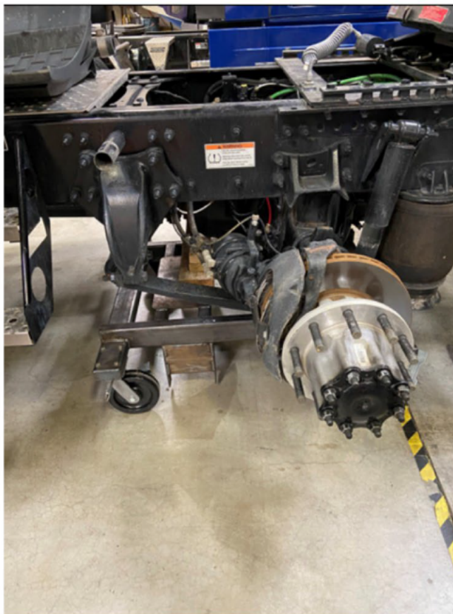
Fig. 1, Resting the Axle on the Dolly
