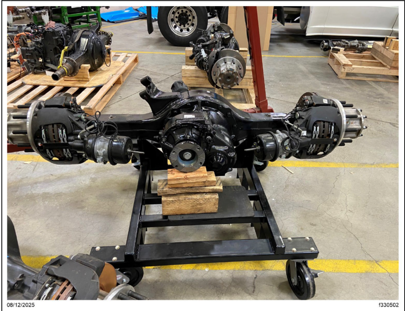
Fig. 4, Axle Removed from the Chassis
