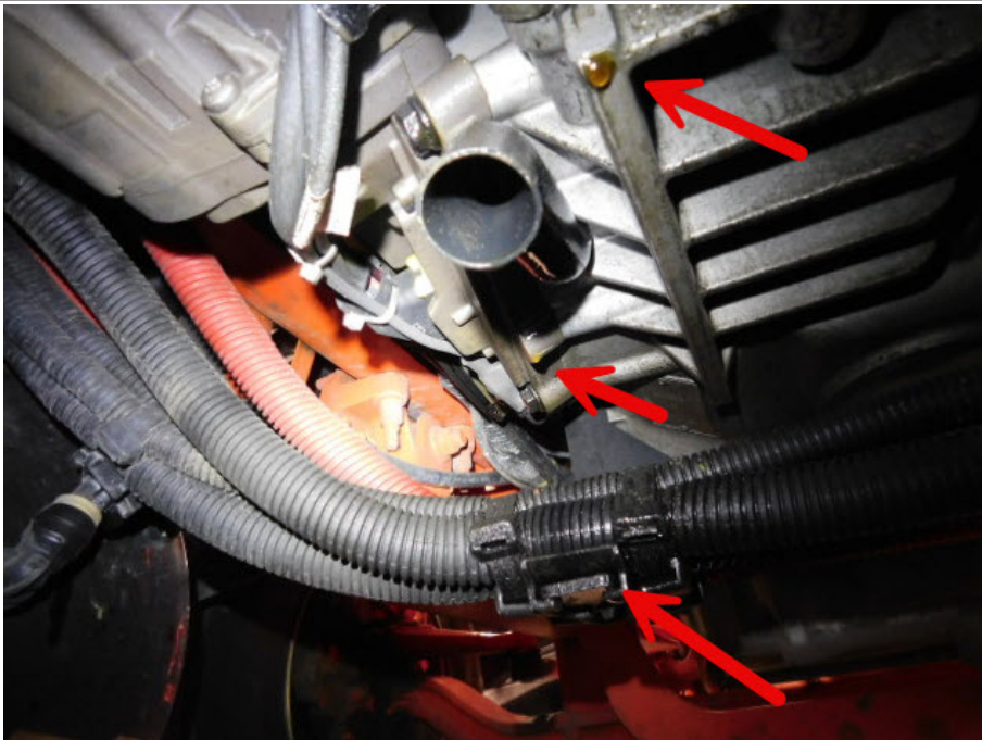
Figure 7 - Oil Leak at the ECA
