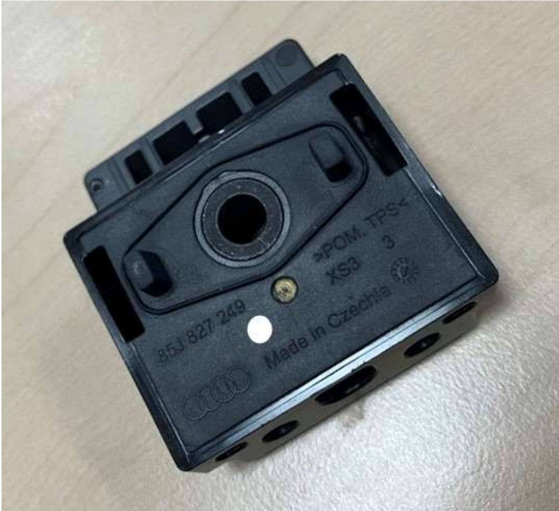
Figure 1. Example of an acoustic buffer with optimized spring without index A marked by a white dot.
