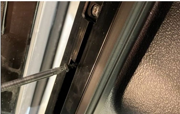
Step 15- Insert Screw At An Angle To Hold Sensor In Place. (You Can Also Super Glue)
