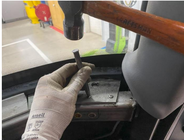
Figure 4: Punch rivets into the structure
