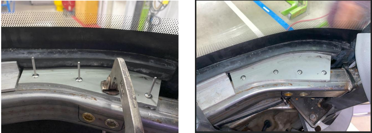
Figure 7: Secure support plate with 3/16" size SST rivets
