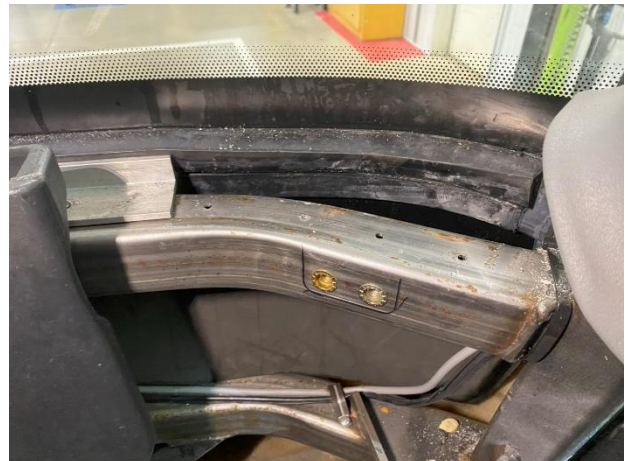
Figure 5: Support plate is removed
