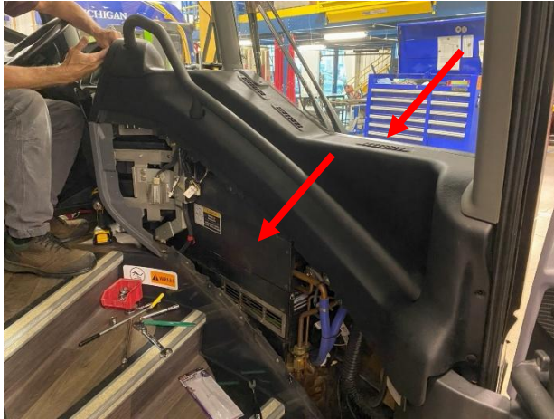
Figure 2: Remove interior components to get access to the windshield support frame
