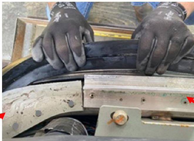
Figure 8: Pull seal off from the joint area
