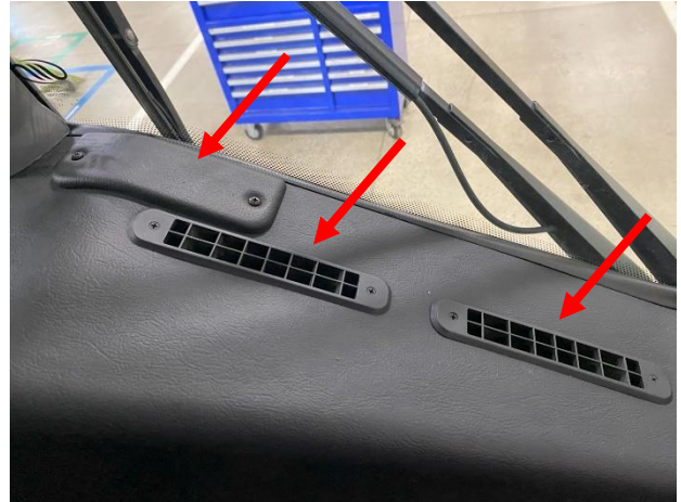
Figure 2: Remove interior components to get access to the windshield support frame
