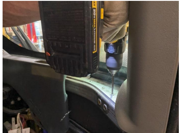
Figure 3: Drill out the head of the rivets
