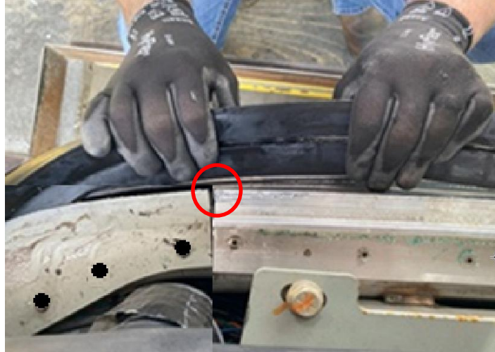
Figure 9: Align inner corner of the side plate with the center profile
