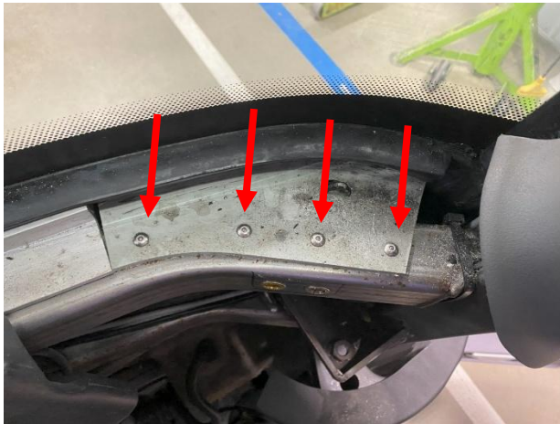
Figure 3: Drill out the head of the rivets
