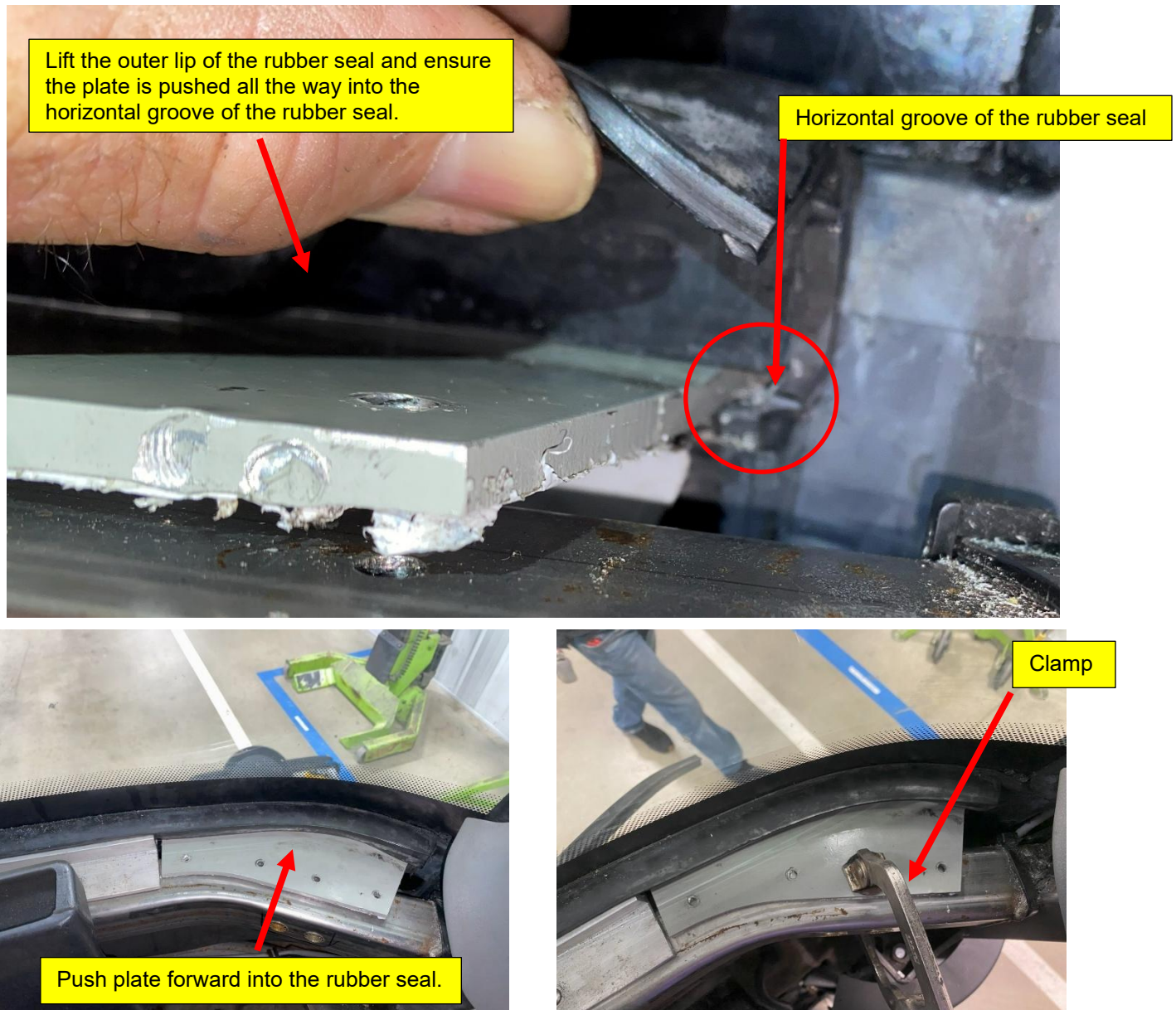
Figure 6: Push plate forward, into the slot of the rubber seal
