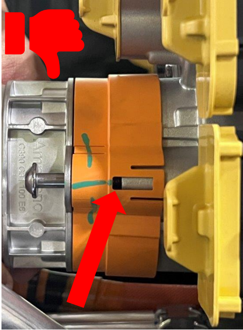
Not Good: Air Gap in Window
