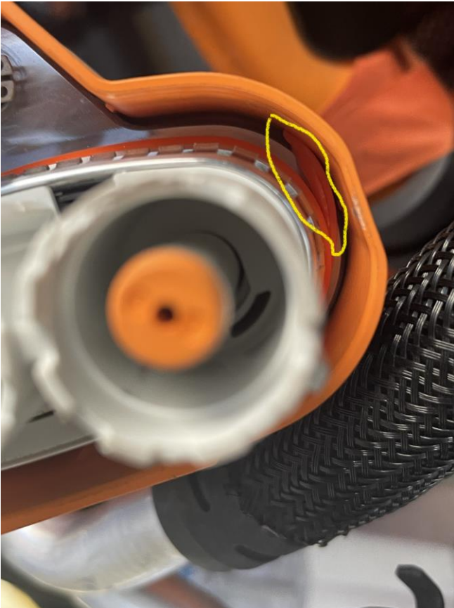
Damaged HV Connector Seal
