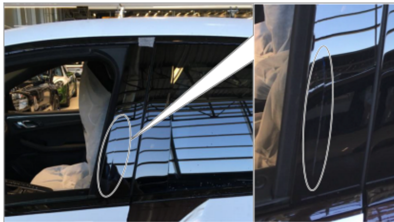
Cracking on B-pillar cover
