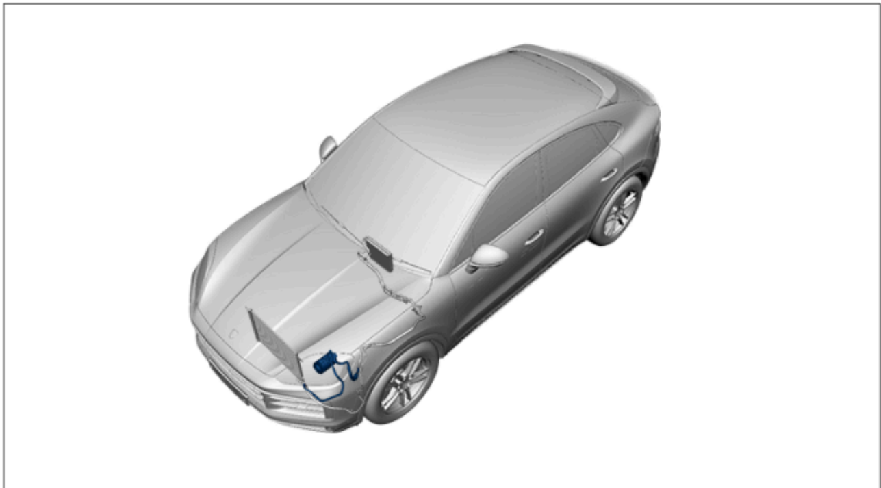
Installation location for air-conditioning compressor / refrigerant lines (shown on the Porsche Cayenne)
