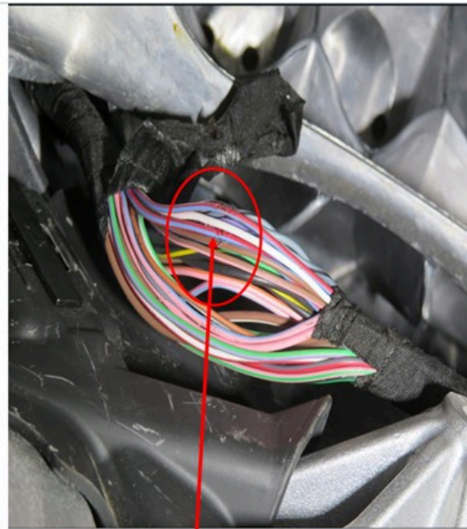
Wiring harness cut near rear e-ATS
