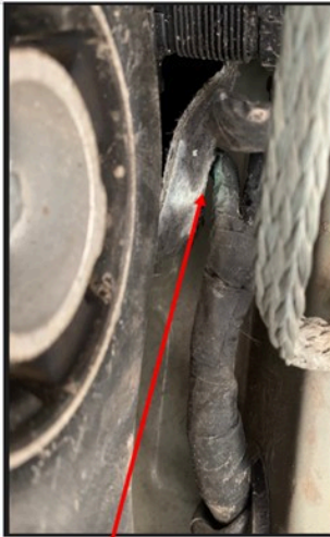
Twisted harness | Harness scratching with the body
