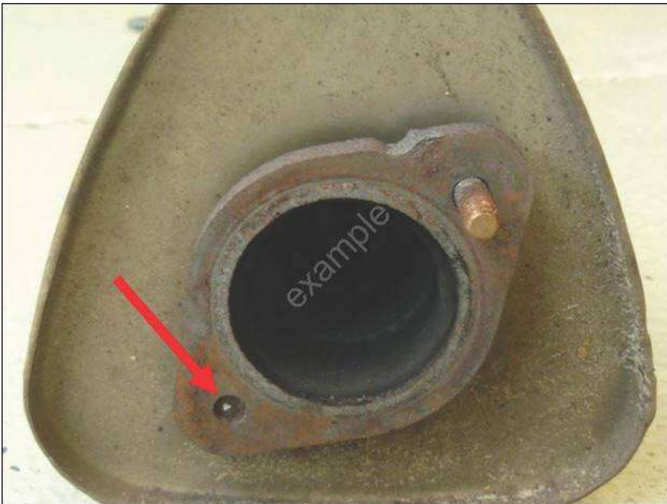
Figure 1. Example of torn-off stud on front silencer (red arrow).
