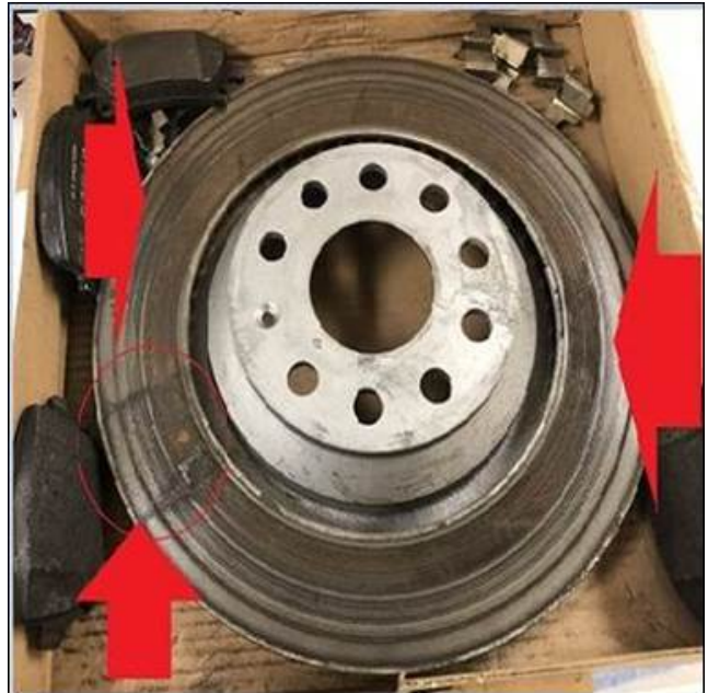
Figure 6: Corrosion, brake pad stuck to brake rotor.
