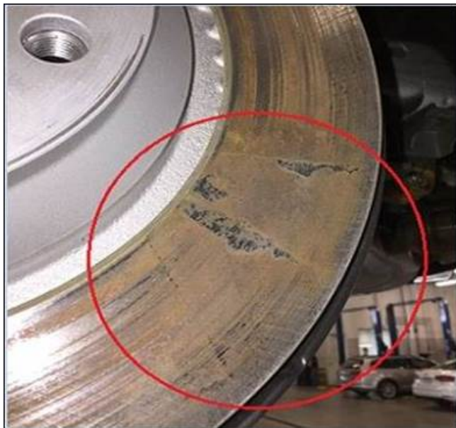
Figure 7: Corrosion, brake pad stuck to brake rotor.
