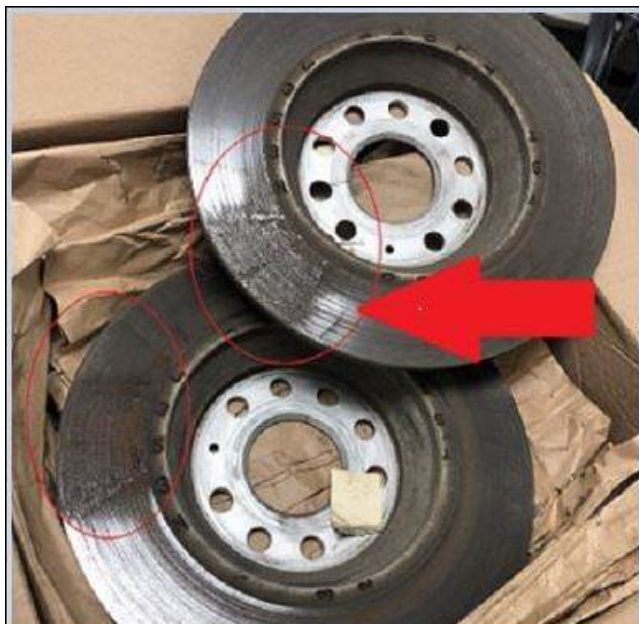
Figure 7: Corrosion, brake pad stuck to brake rotor.
