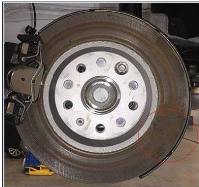
Figure 8: Corrosion, brake pad stuck to brake rotor.
