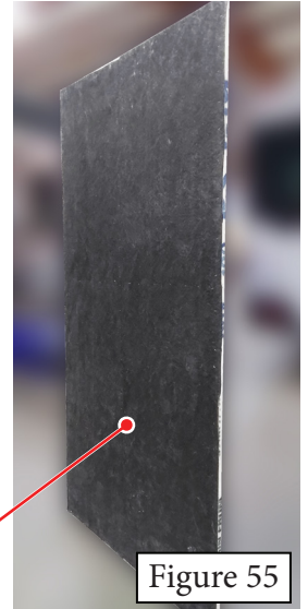
FELT COVERED PLYWOOD
