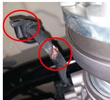
Figure 3 - Cable damaged and clip disconnected
