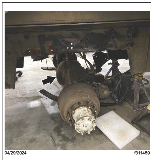
Fig. 7, Rear Axle Removed from the Vehicle
