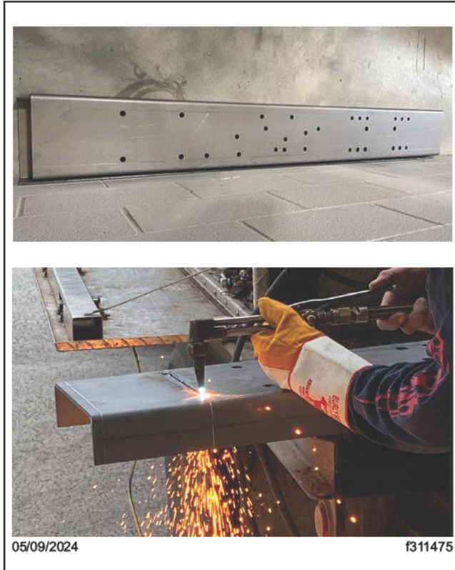
Fig. 33, Cutting the New Frame Rail to the Required Length
