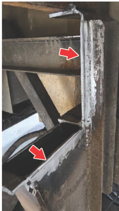
Fig. 31, Old Weld Cleaned and Prepared for the New Frame Rail Installation
