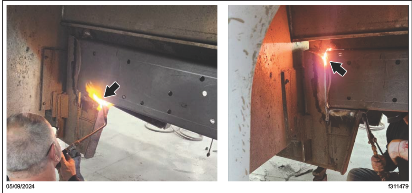
Fig. 37, Preheating to 150-Degree Fahrenheit
