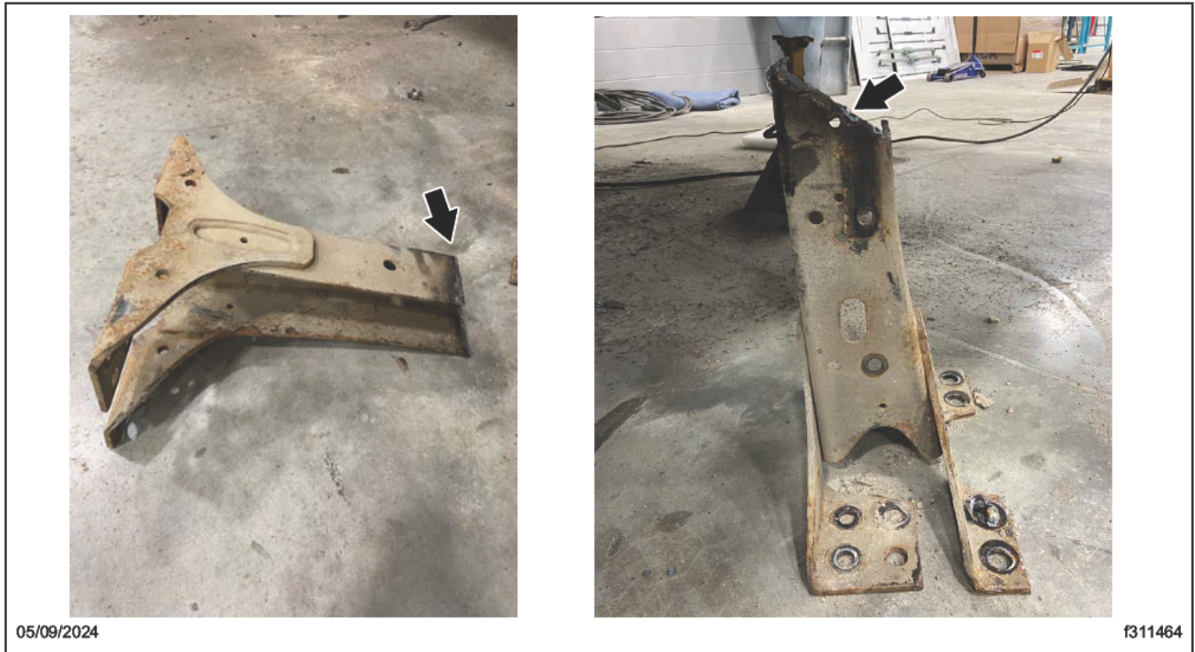
Fig. 18, Crossmember Cut at a 45-Degree Angle
