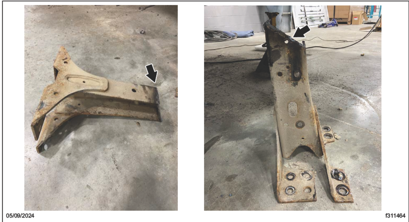
Fig. 24, Crossmember Cut at a 45-Degree Angle
