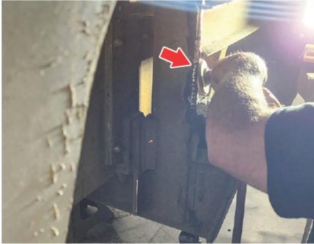
Fig. 30, Grinding the Cut Areas
