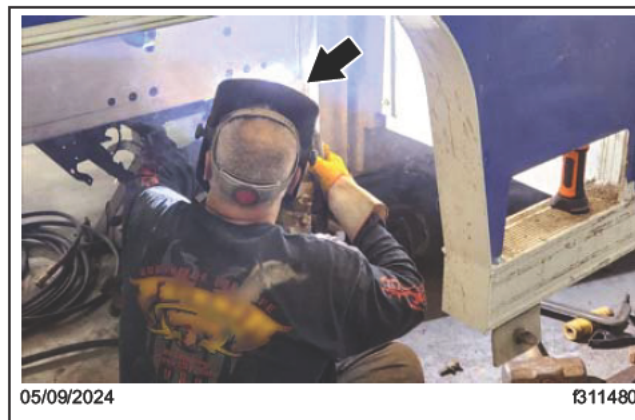
Fig. 38, Laying the Final Weld
