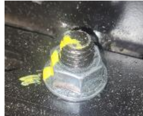
Figure 13: How a torque mark must be applied.
