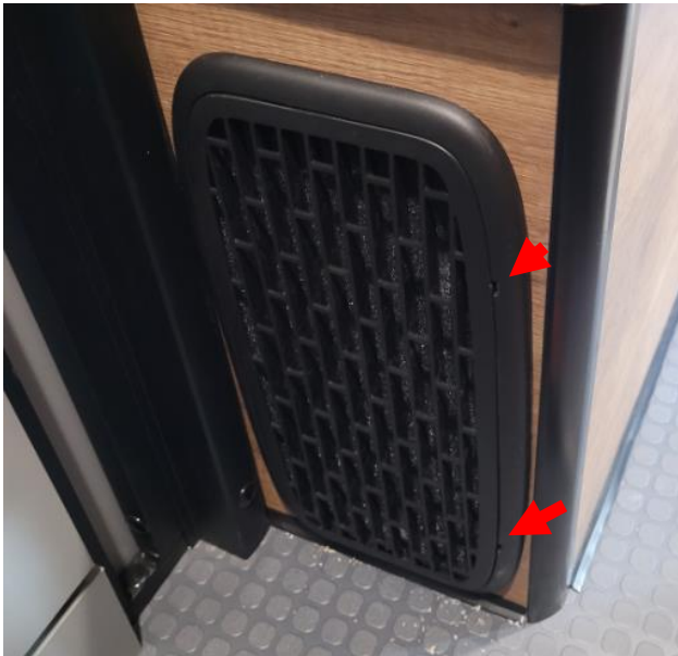
Figure 8: Plastic cover, red arrows are pointing to slots
