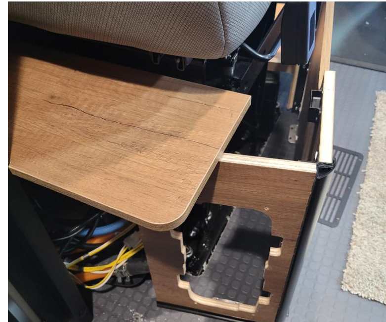
Figure 11: Dinette seat cabinetry is now loose.
