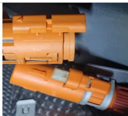
Improperly connected HV connectors
