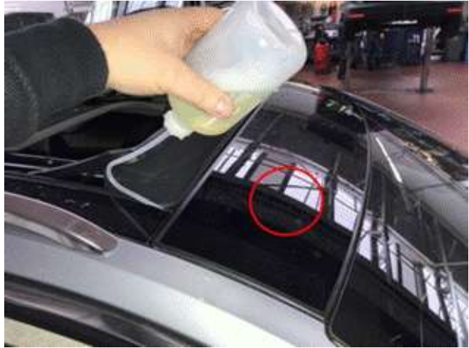
Figure 11. Rinsing the drainage channels.
