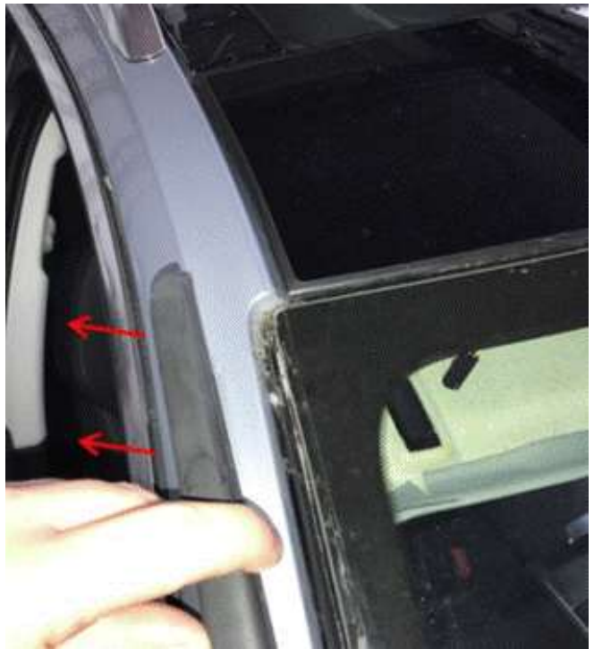
Figure 6. Water deflector removed.
