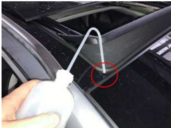
Figure 10. Rinsing the drainage channels.
