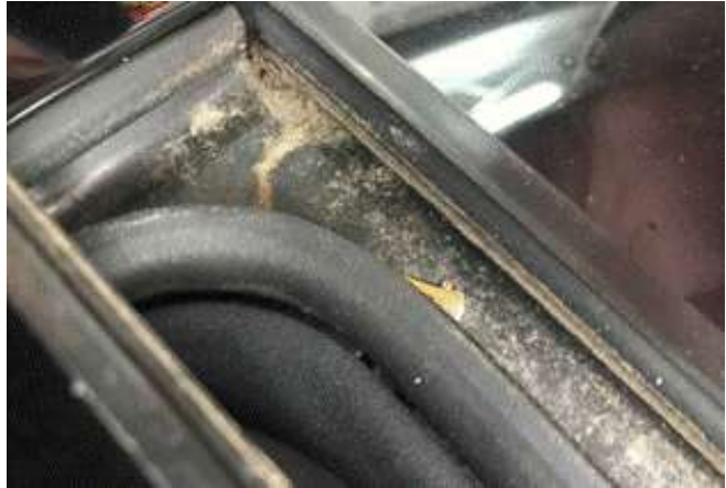
Figure 2. Dirt in the front sunroof frame.
