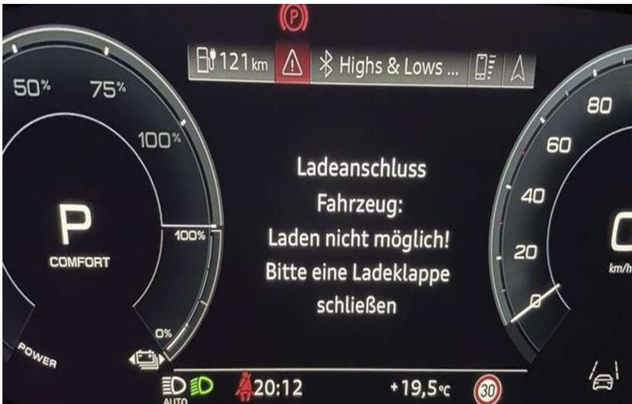
Figure 2. “Vehicle charging port: charging not possible! Please close the charging flap” (example).
