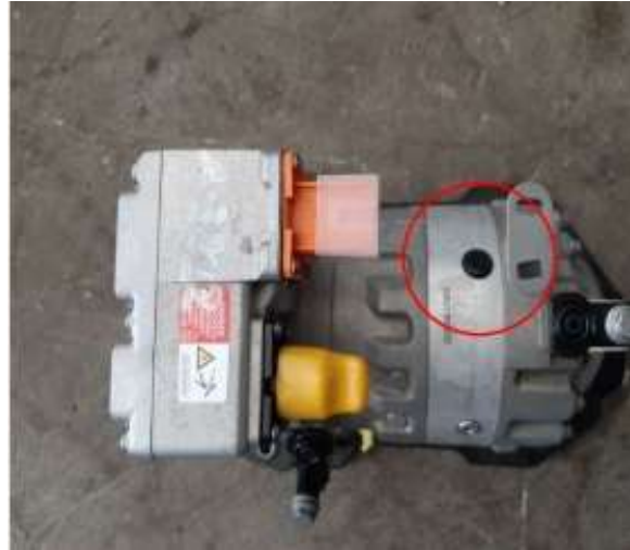
Figure 1. Pressure relief valve on the air conditioning compressor.
