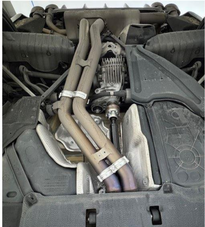
Figure 1. Bottom View of the exhaust system with clamps installed
