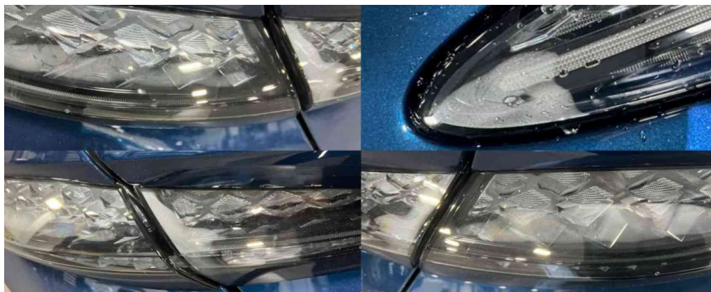
Figure 1b – Rear tail lights steamed up/damp from the inside with minor drips
