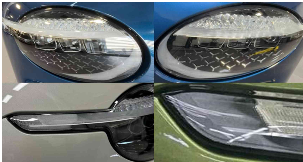
Figure 1a – Front headlights steamed up/damp from the inside with minor drips
