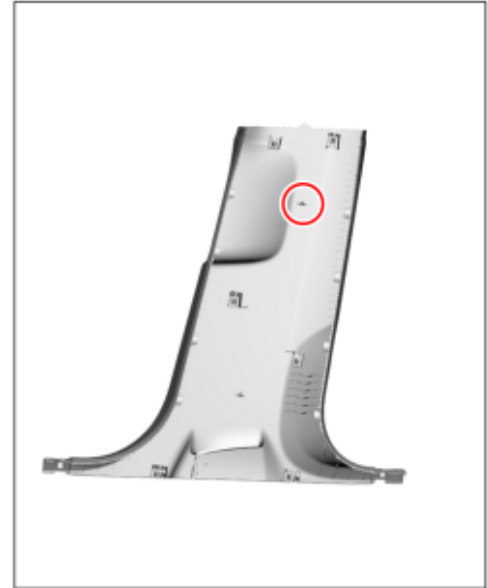
Enclosure: Material contact point of B-pillar trim panel (lower part) on the left
