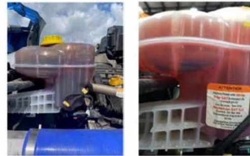
Examples of discolored surge tanks
