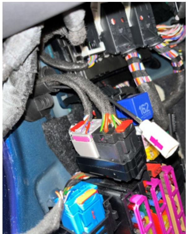
Figure 11 Door Harness Connection Point (2)
