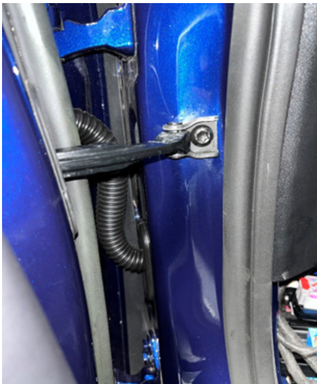
Figure 10 Door Harness Connection Point (1)
