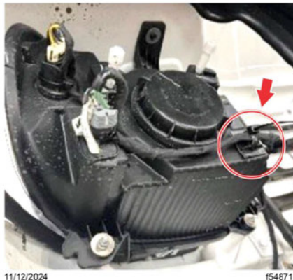
Fig. 1, Stick-On Cable Tie Attached to Headlight Housing
