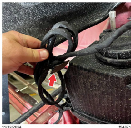
Fig. 1, Stick-On Cable Tie Attached to Headlight Housing
