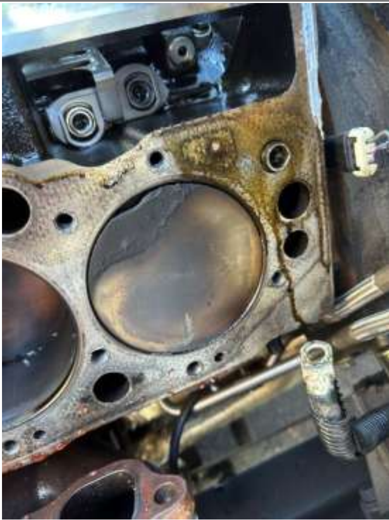
Example of a melted piston.
