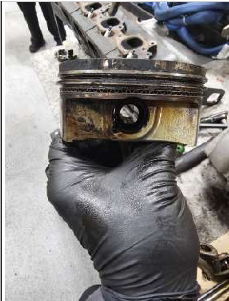
Example of carbon buildup causing the piston rings to stick, creating blowby.
