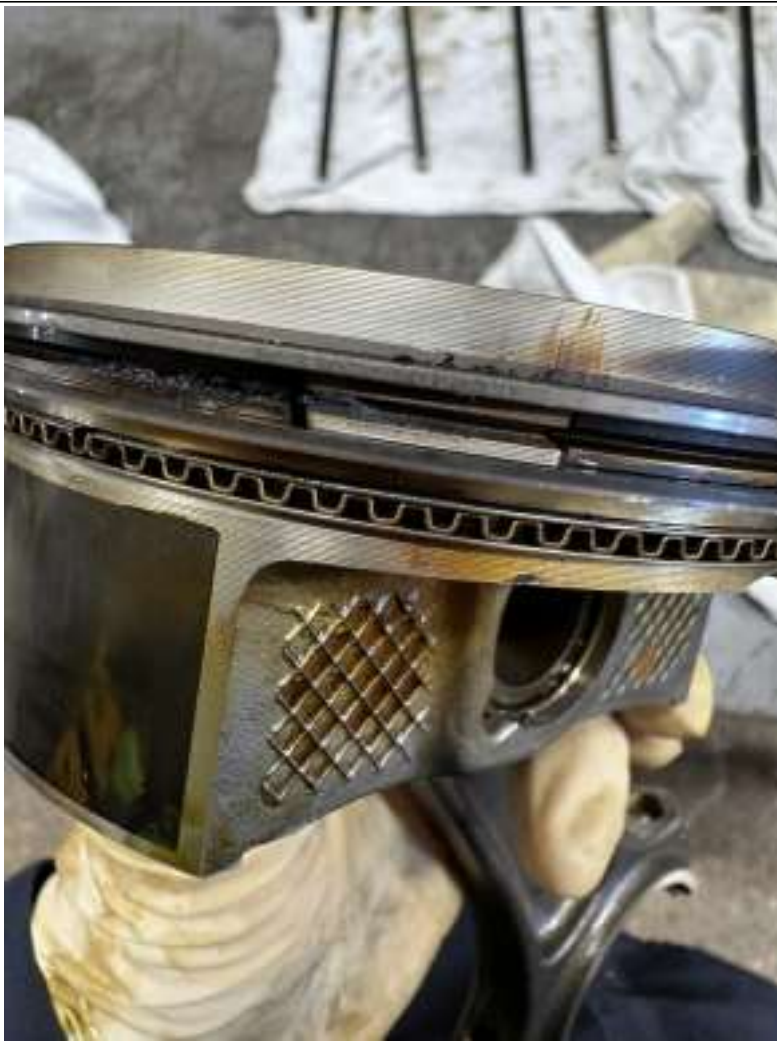
Example of a broken compression ring.
