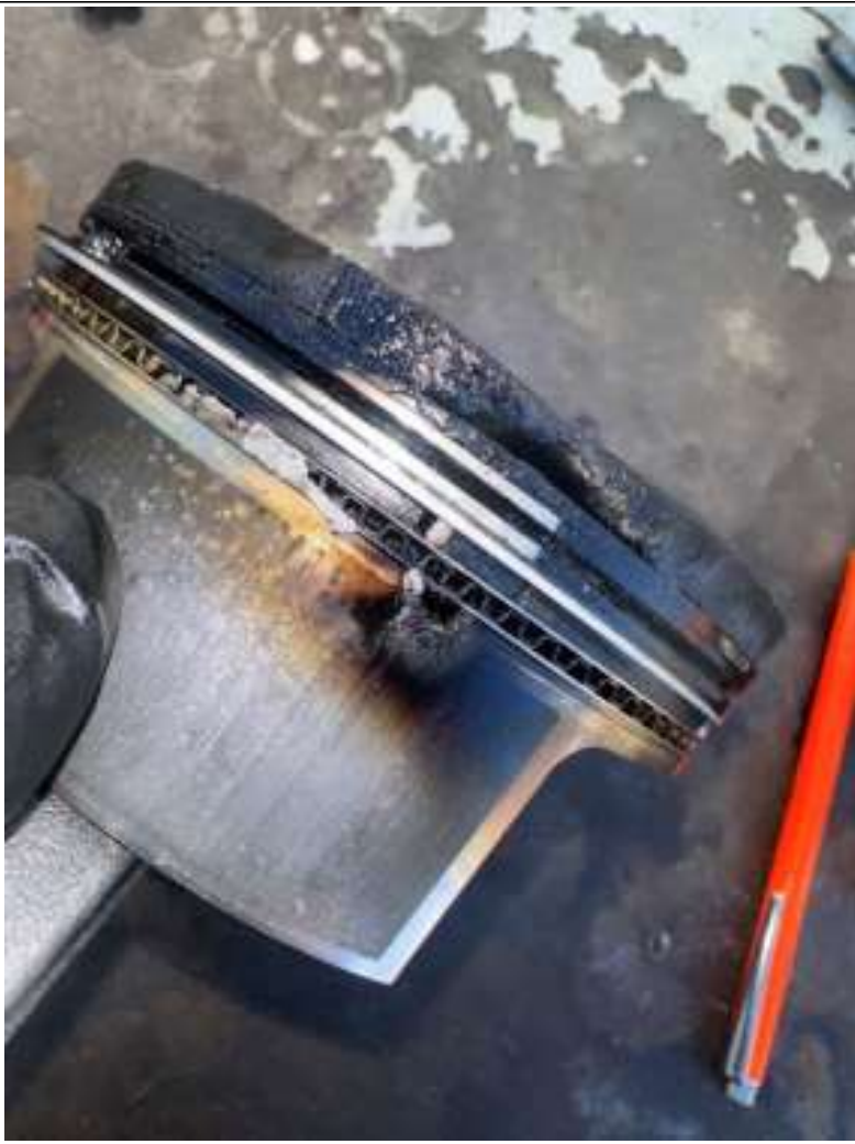
Example of a burned piston with metal in the oil control ring.
