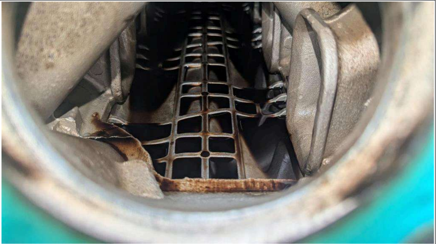
Example of oil pooling in the intake manifold.
