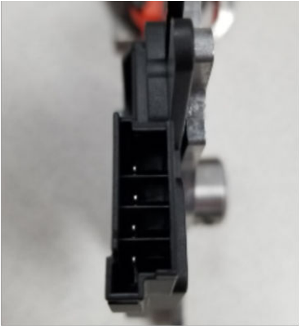
Example of a 4 pin internal harness connector.
