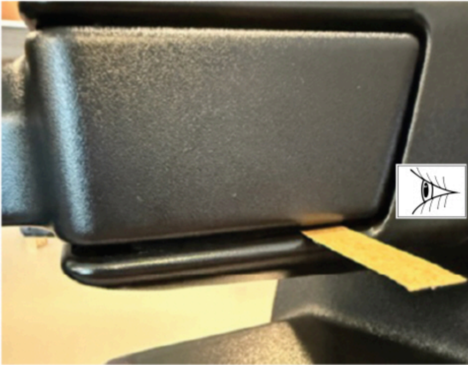
Figure 4 – incorrect flock tape application
