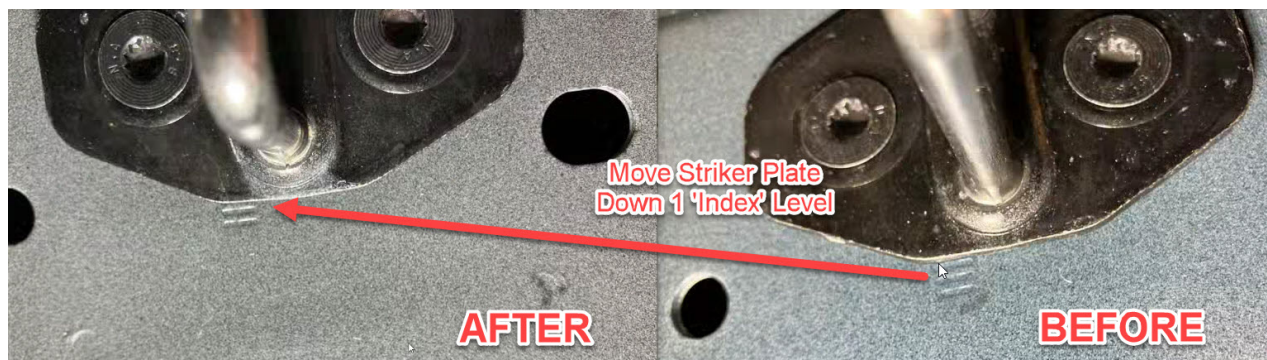
Figure 2 - Rear locking bar 'index' level adjustment
