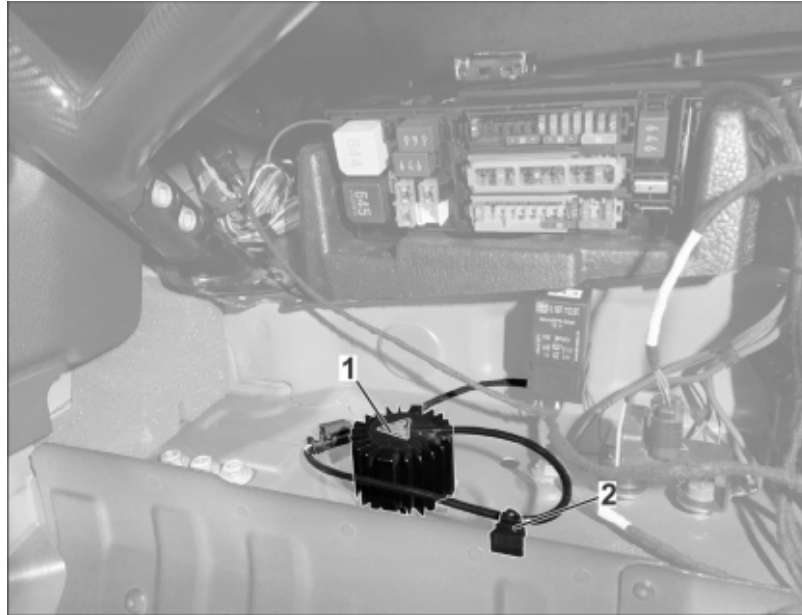
Installing rear right resistor
