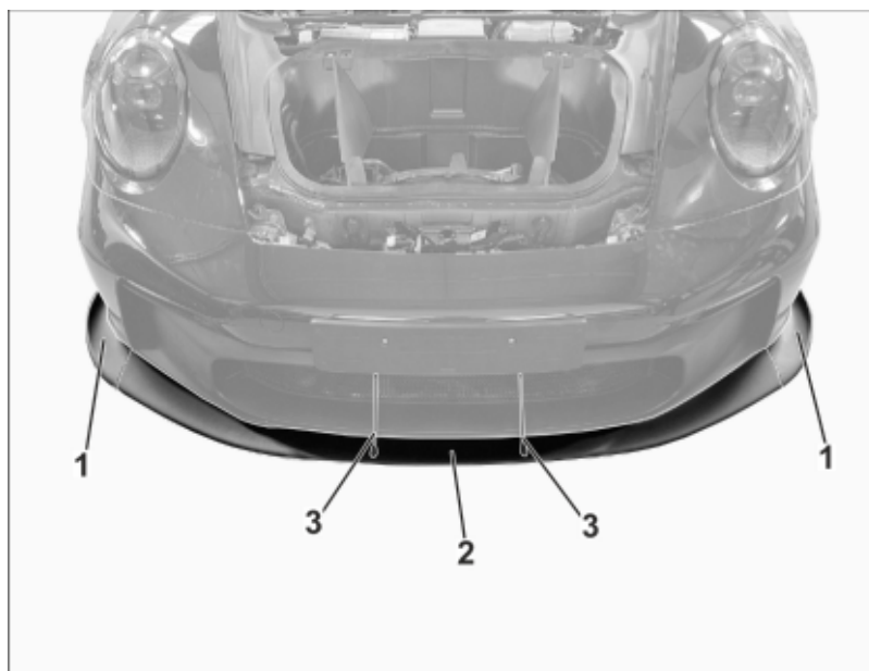
Assembly of front lips and front lip rods
