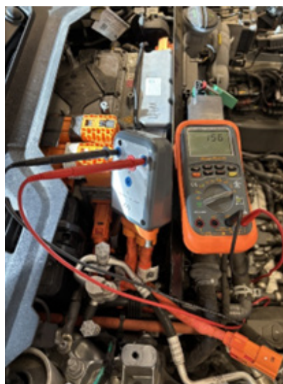
Figure 3 - Measuring Capacitance on Front PE
